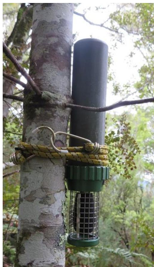
**Figure 2: KLD attached to narrow tree with bungee cord**
