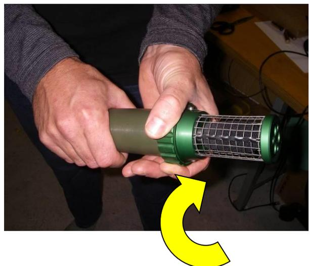
Avoid excessive force on the mesh microphone cover (if the locking ring is tight then grip the tube while removing it – not the microphone cover).
